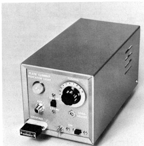
Exterior view of the 15-watt transmitter. All controls are located on the front panel.
